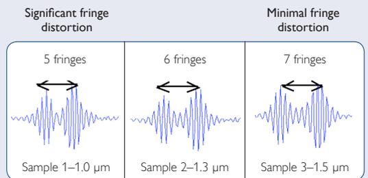
Fringe distortion increases significantly for film thicknesses below ~1.5  $\mu\text{m}$ . This has the effect of displacing the peaks, making it impossible to establish the true thickness of the film using traditional Thick Film Analysis
