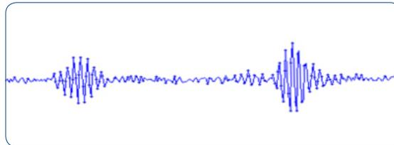
The thickness of the film can be determined by locating the positions of the two maxima and applying the refractive index. In addition, the surface information of the two interfaces (air/film and film/substrate) can be obtained from the individual fringes (Figure 5).
