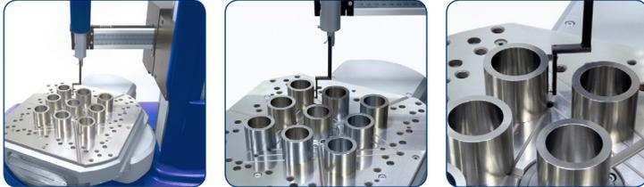
A **critical** component for the compressor is the crank, manufactured again to a high specification this offset is essential to the operation of the compressor; this feature has not been possible to measure in the past due the large offset, however with the large movement of the XY stage, several can now be mounted at one time and this offset can now be measured and quantified, an important advantage of the TalyMaster stage.
