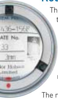
The glass hemisphere is a high precision standard used to both calibrate and evaluate the performance of roundness measuring instruments.
